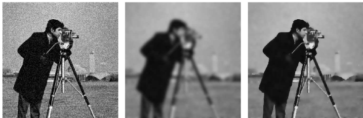
Figure: Left: Original cameraman image. Middle: Noisy image(random noise). Right: Denoising by linear diffusion. Bottom right: Denoising by Perona-Malik nonlinear diffusion. Parameters: 25 iterations, t = 0.15 .
